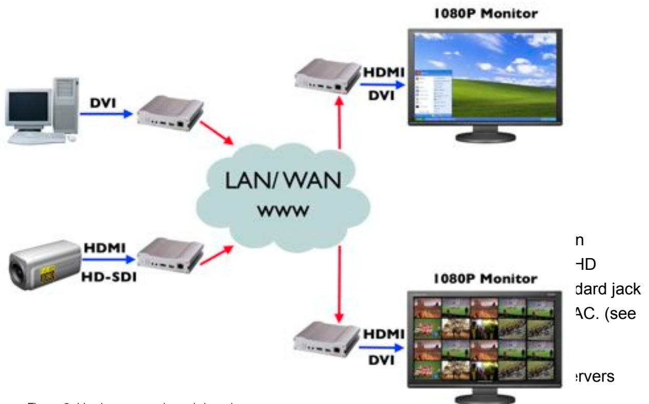
Figure 2: Hardware encode and decode
